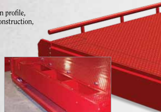
End cleanout area
